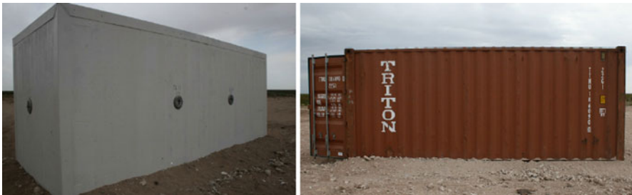
Fig. 13.12 Live explosive test specimens: blast-resistant module ( left ) and standard ISO container ( right )
