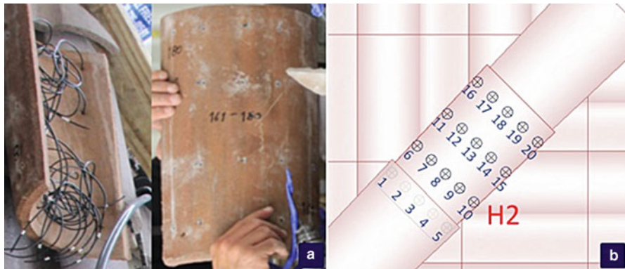
Fig. 17.4 Pressure taps layout. (a) Hip/ridge tile with installed pressure taps. (b) Numbering of pressure taps (Baheru et al. 2014a)
