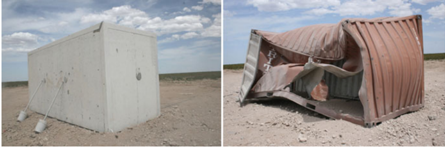
Fig. 13.15 Blast-resistant module and ISO container after live explosive testing with 4,000 kg of ANFO at 46 m. BRM experienced less than 1 cm (0.4 in) of permanent deformation
