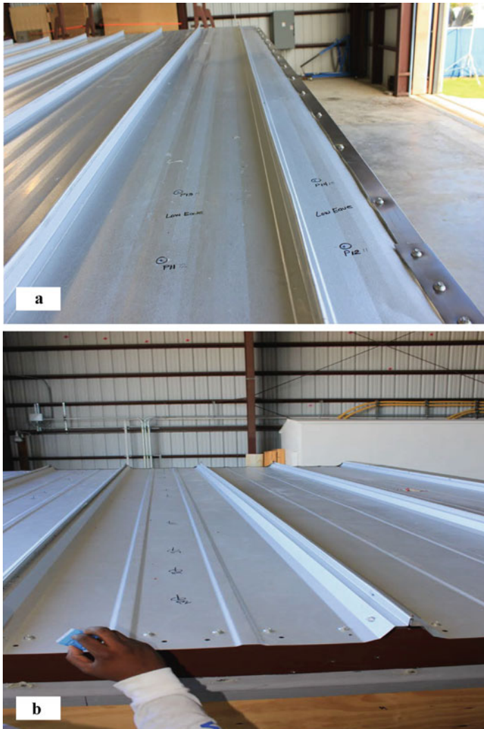
Fig. 17.10 Standing seam metal roof mock-ups used in testing: (a) vertical-leg and (b) trapezoidal roof
